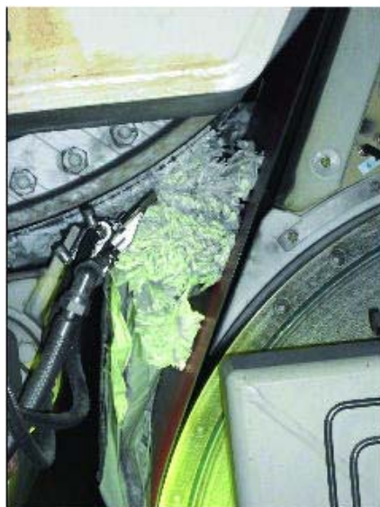
Fig. 5: View of a "hidden" blade in a press section
