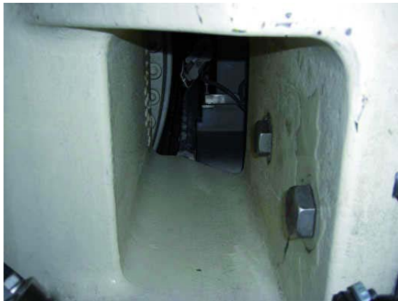
Fig. 5: View of a "hidden" blade in a press section
