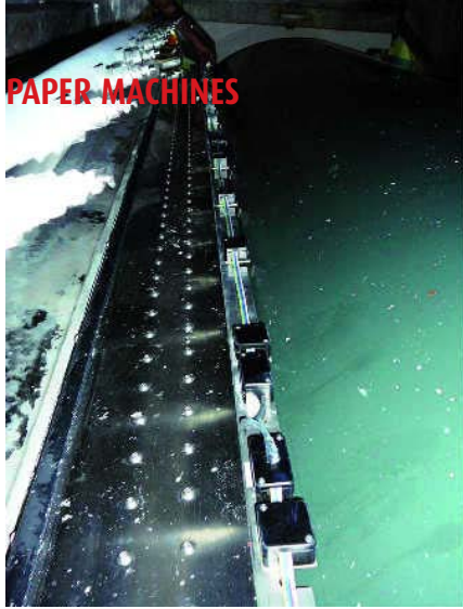
Fig. 4: View of a BladeCheck™ measuring device in action
